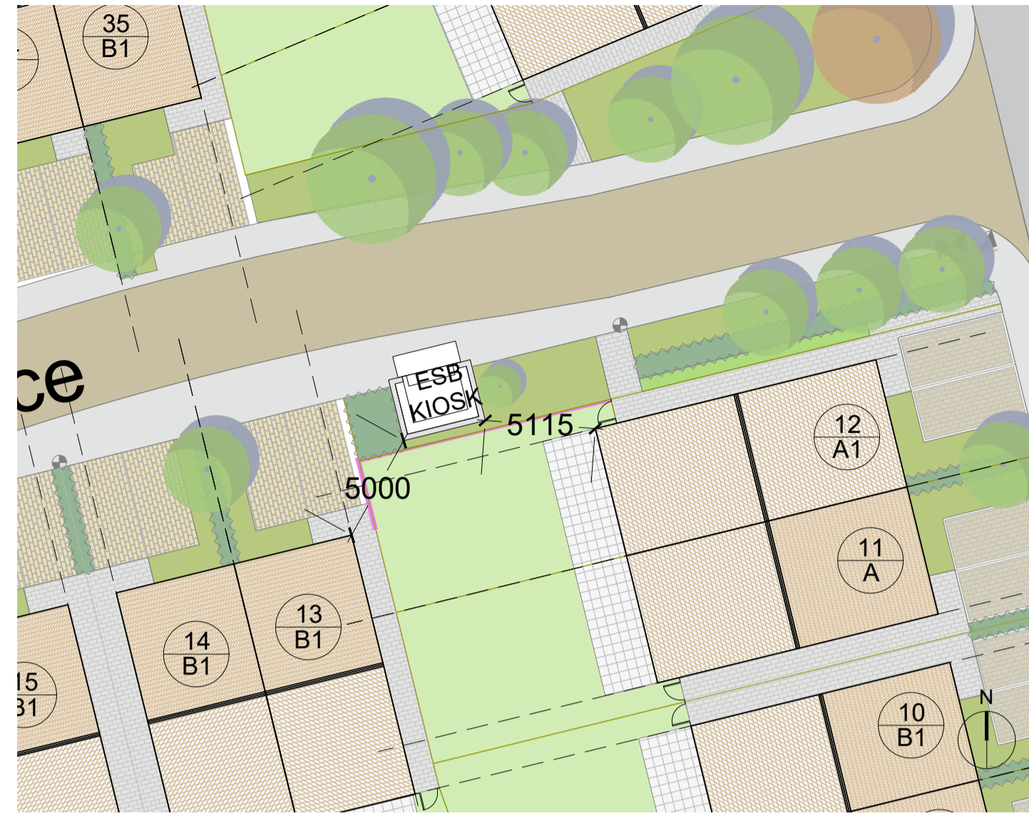
LOCATION PLAN - Sub station Kiosk 02- Scale 1: 250
